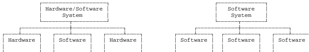
FIGURE 13. Two types of systems handled by MIL-STD-498.
